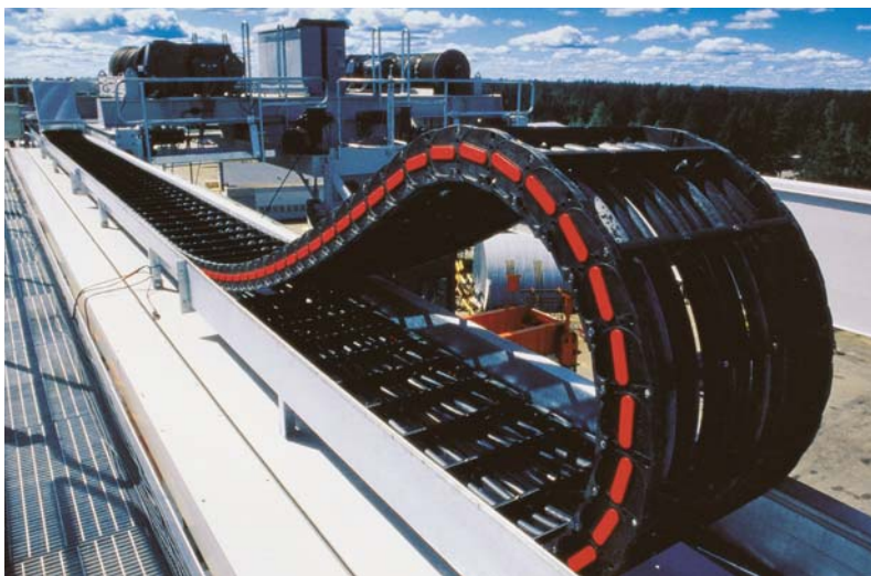
Typical single-loop power chain installation on a KCI Konecrane RTG unit in operation
