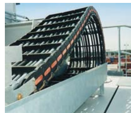
Typical single-loop power chain installation on a KCI Konecrane RTG unit in operation
