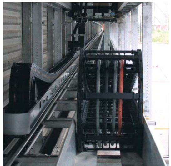
Chain/Cable testing rig for long travel: Tests at 8 m/s for 130 m travels.
